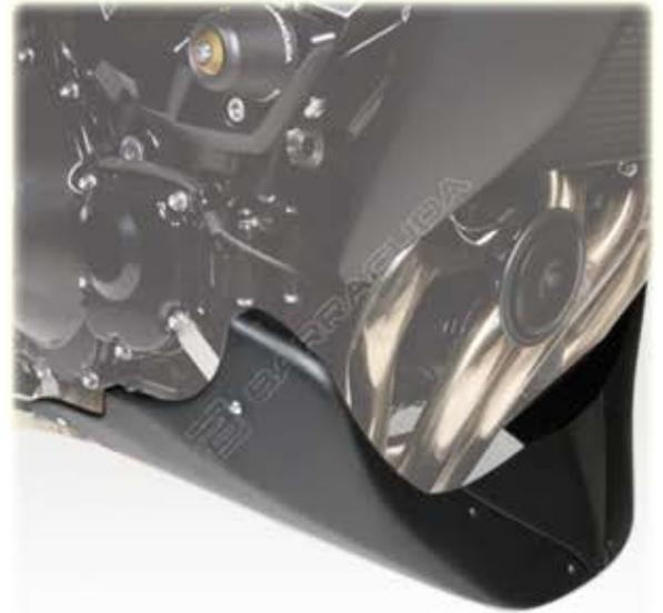
FIX THE ABS ENGINE SPOILER WITH ITS SCREWS KIT 4X10, WASHERS AND NUTS.
